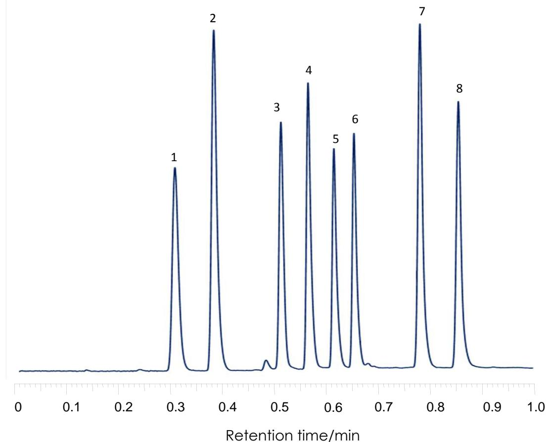
Column: SunShell C18 2.6 µm, 30 x 3.0 mm.
