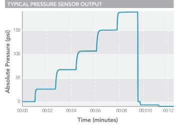
This graph shows the overlaid output from ten pressure sensors monitoring the same fluidic channel. High reproducibility and the capability for simultaneous reading of multiple sensors make the units extremely valuable for instrumentation applications. In this plot, the sensors are responding to a series of pressure increases over the sensor range.
