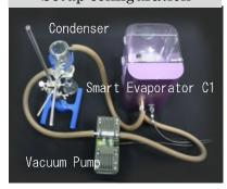
\* Insert the hose nipples to the ports on the back of the Smart Evaporator C1 and inlet/exhaust ports of the vacuum pump.
