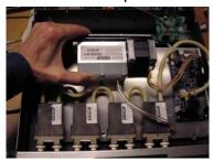
2: Secure the new tray using 1 M3 x 6 and 2: M3 x 16 screws saved earlier.
