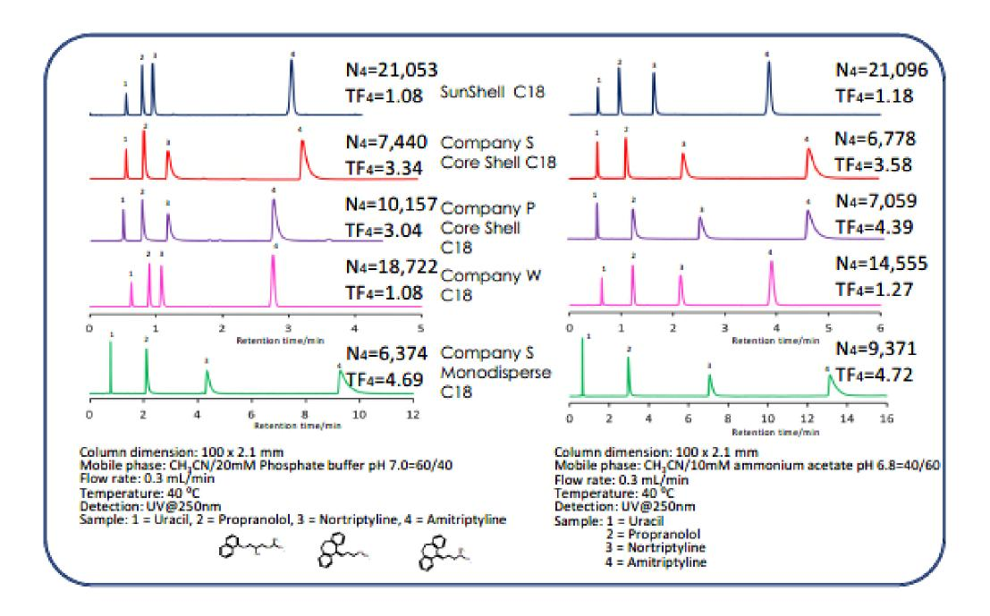
Amitriptyline was used as a basic compound and two kinds of mobile phases were used. SunShell C18 showed the best peak shape and the highest theoretical plate for a basic compound like amitriptyline.
