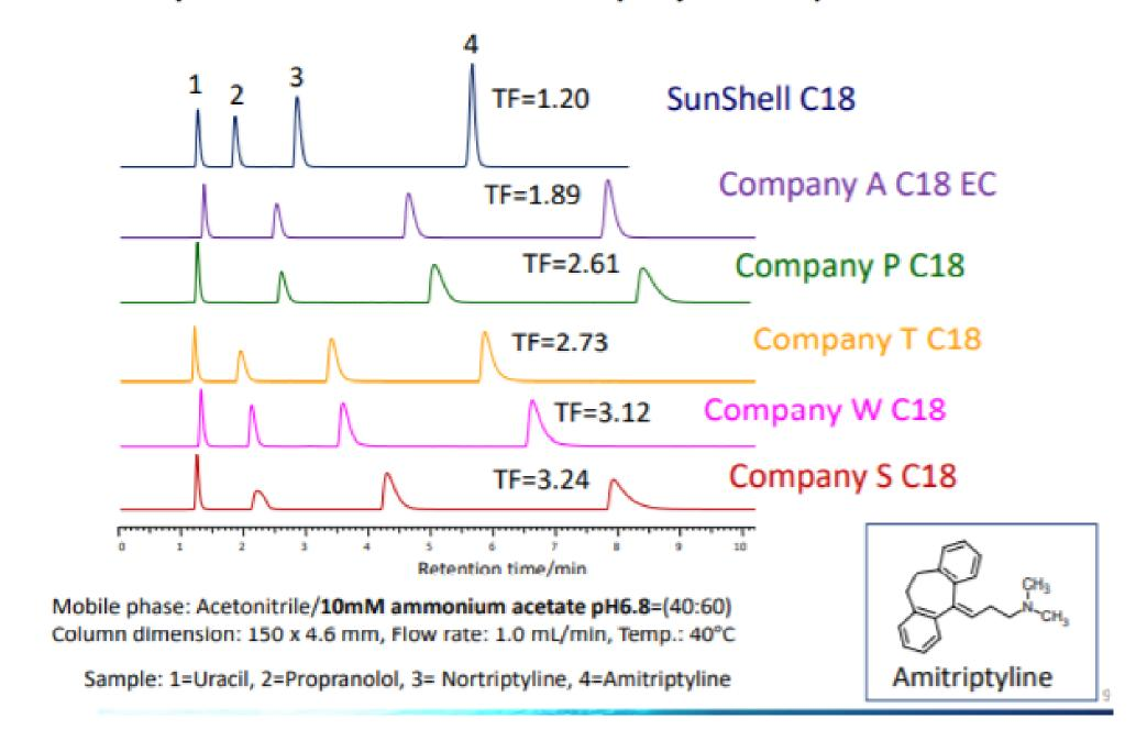
This slide shows a comparison of amitriptyline peak using acetonitrile and 10mm ammonium acetate mobile phase. SunShell C18 showed a good peak shape. The SunShell column also showed the least amount of Tailing Factor (TF) as highlighted above.
