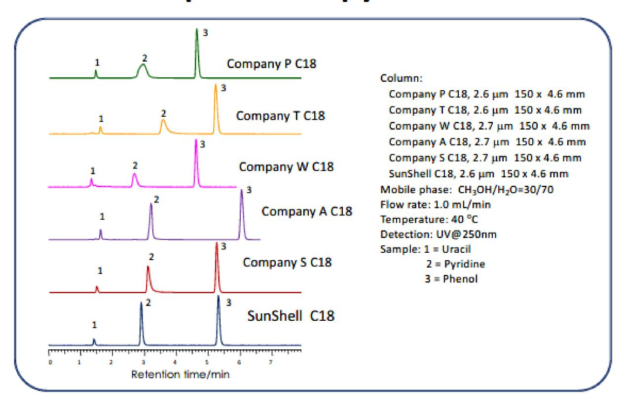
Pyridine peak shape was compared and the effect of residual silanol groups was evaluated. Mobile phase is methanol and water 30 to 70. Number 2 peak is pyridine. SunShell C18 showed a good peak shape. However Company P Kinetex C18 and company T Accucore C18 showed a bad peak shape.
