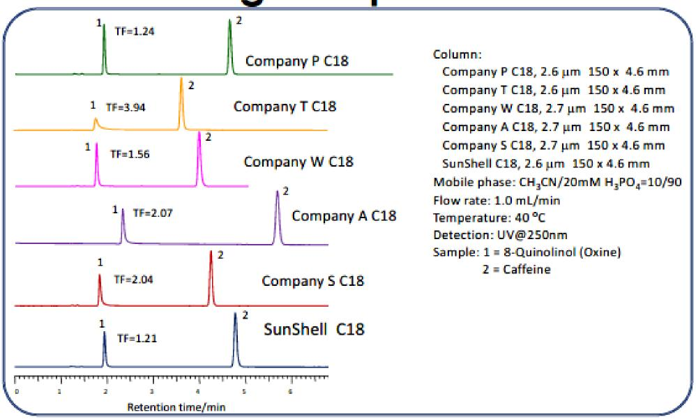
8-quinolinol, a Oxine peak shape (peak number 1) was compared with other columns. The amount of metal impurities in the core shell silica was evaluated because oxine is a metal chelating compound and the metal impurity causes oxine to peak tail. SunShell C18 had the best peak shape with the least amount of tailing compared to the other columns in the analysis.
