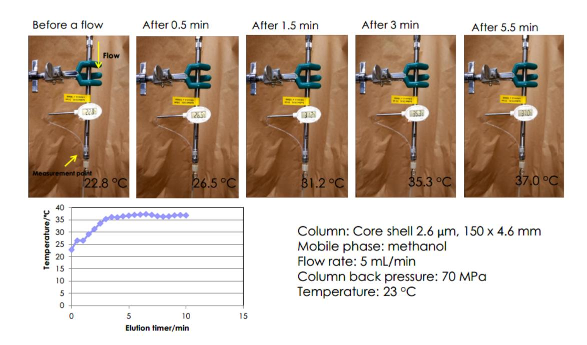
We measured the temperature of the surface of the column outlet when methanol flowed at 5 ml/min at 70 MPa
