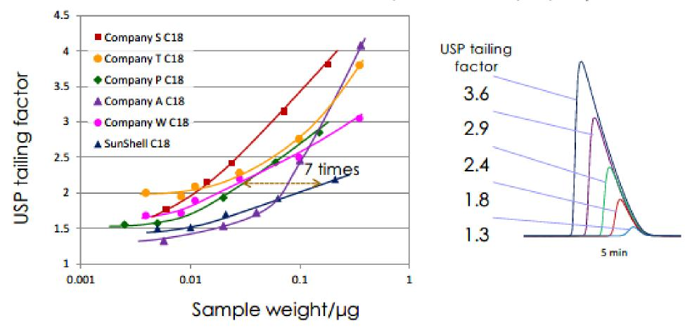
In the case of using acetonitrile /0.1% formic acid as a mobile phase, amitriptyline peak shows more tailing because a loading capacity decreases in an acidic, low-ionic-strength mobile phase.
