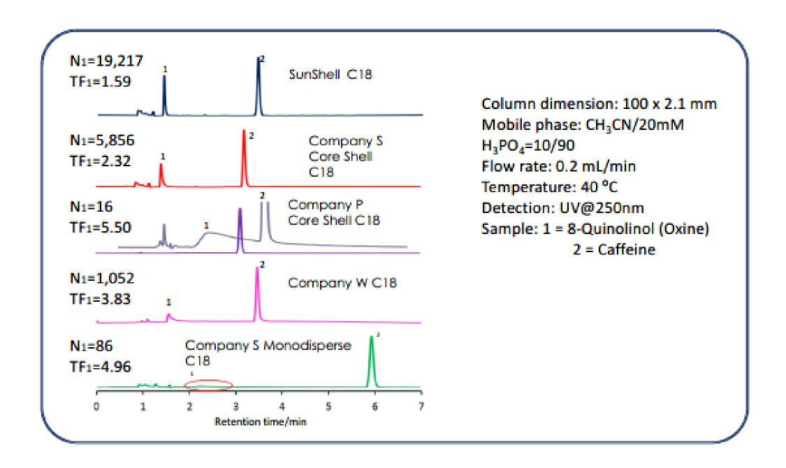
Oxine is a metal chelating compound. It is considered that Company P and Company S shows a low theoritical plate number and tailing. This means that they have a lot of metal impurities
