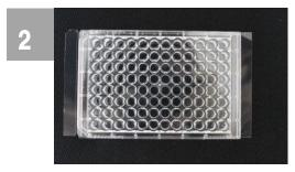
Apply the adhesive side of the sealing sheet to the plate.
