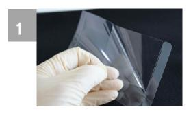
Peel off the separation film using a slit to expose the adhesive side of RAPID CRS.
