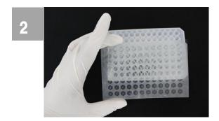
Paste the RAPID SlitSeal on the 96-well plate and make sure holes of RAPID SlitSeal are correctly positioned on each well spot.
