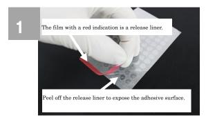
Remove the release liner with a red indication and expose the adhesive surface.
