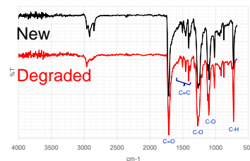
Figure 1. FT-IR spectra: New/Degraded products, PBT
