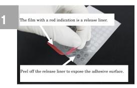
Remove the release liner with a red indication and expose the adhesive surface.
