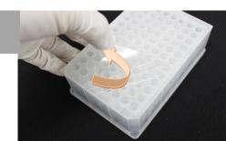
Remove the protective film before sampling or dispensing. If used without removing the protective film, the needle or the tip can not puncture the film. If the protective film stays on and is left at 100°C, the edge of the protective film may be curved.
