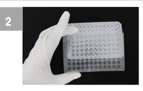
Paste the SUPER SlitSeal on the 96-well plate and make sure holes of SUPER SlitSeal are correctly positioned on each well spot.
