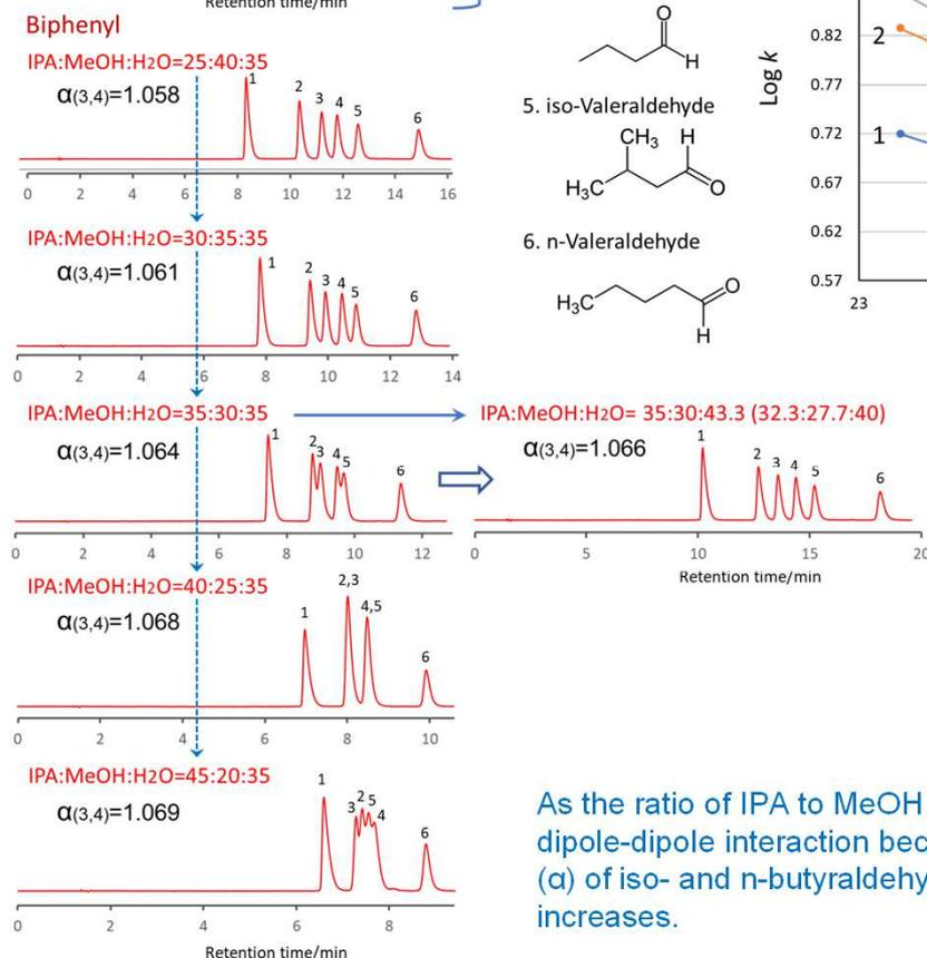
As the ratio of IPA to MeOH in the mobile phase increases, the dipole-dipole interaction becomes stronger and separation factor ( $\alpha$ ) of iso- and n-butyraldehyde-DNPH increases as the IPA increases.
