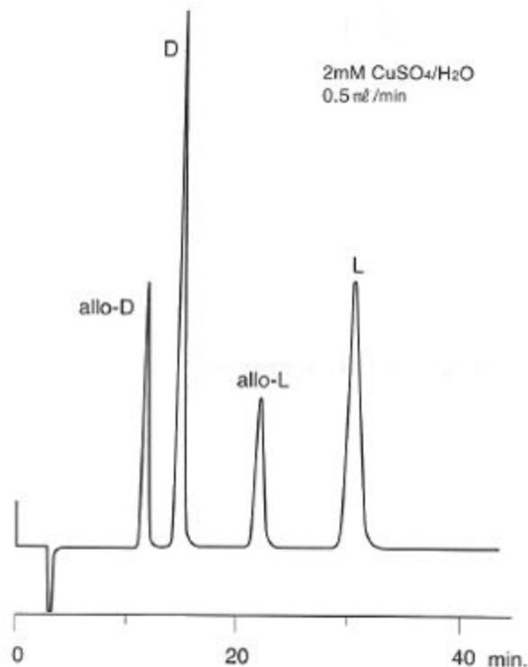
Separation of amino acid mixture on MCI GEL™ CRS10W column.
